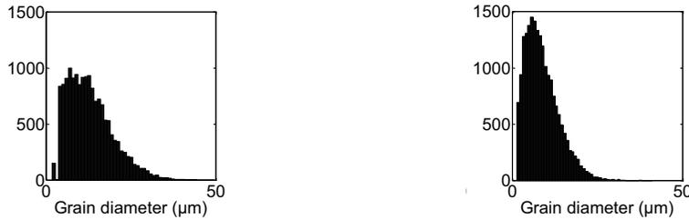
Figure 1. Grain size distribution for finest (right) and largest (left) grain sized IF steel.
