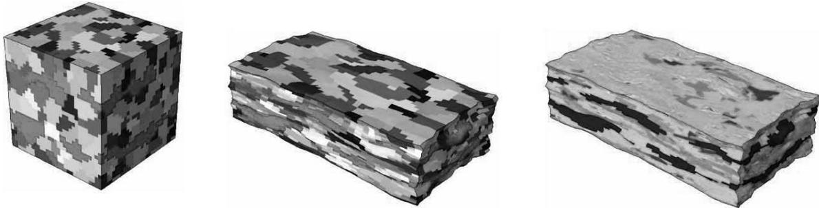
Figure 2: Left: Periodic unit cell model of the generated microstructure. The band-shaped red region represents the pearlite phase. Center: Deformed unit cell model after cold rolling simulation. Right: Von Mises equivalent stress distribution within the unit cell.
