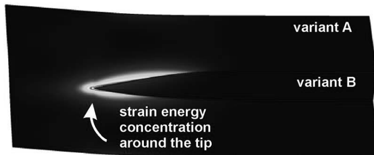
Figure 2. FEM modeling of a martensitic needle of one variant penetrating another variant (two-dimensional model, plane strain, plotted quantity is the strain energy density).
